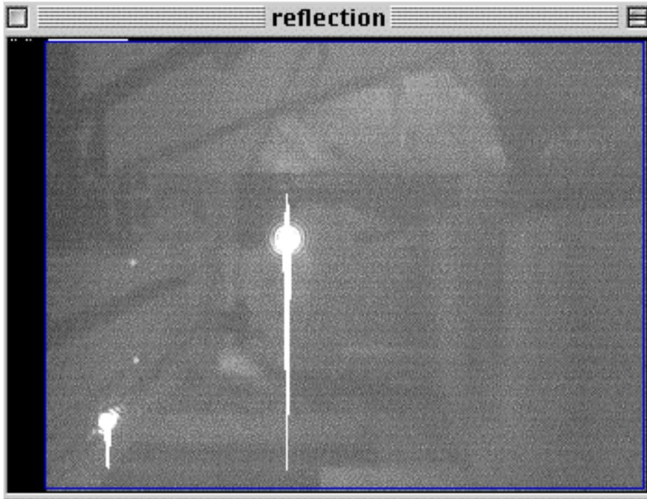
Figure: Reflection in a BCAM Image, 300-ms exposure, with strong intensification. We can see one strong reflection and two smaller ones, in addition to the main image.
