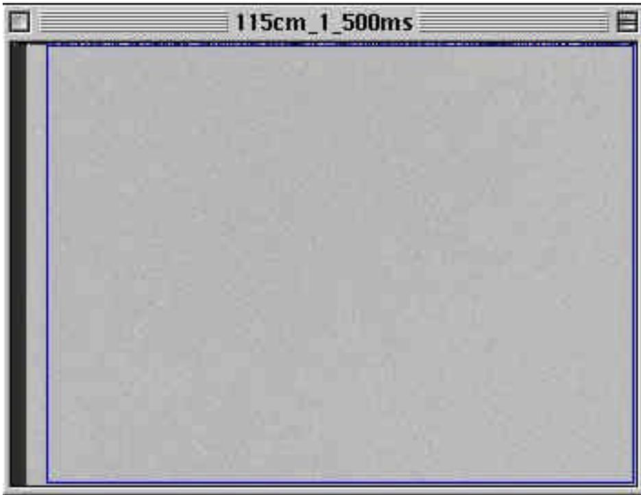
Figure 4: The image captured after 500 ms in the dark by a CCD that had been exposed to 400 Gy. The average intensity is 202 8-bit ADC counts.
