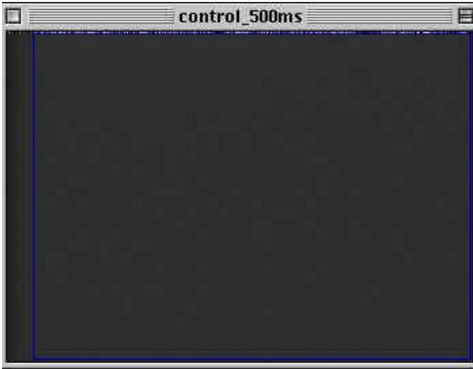
Figure 2: The image captured by an undamaged CCD after a 500-ms exposure with the camera aperture blocked off. The average intensity is 64 8-bit ADC counts.
