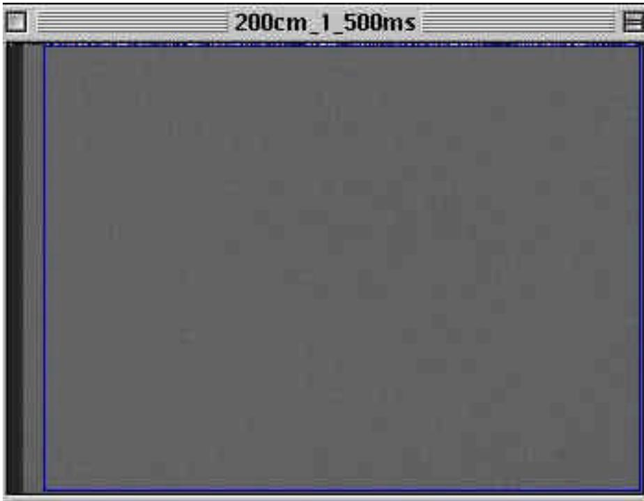
Figure 3: The image captured after 500 ms in the dark by a CCD that had been exposed to 130 Gy. The average intensity is 102 8-bit ADC counts.
