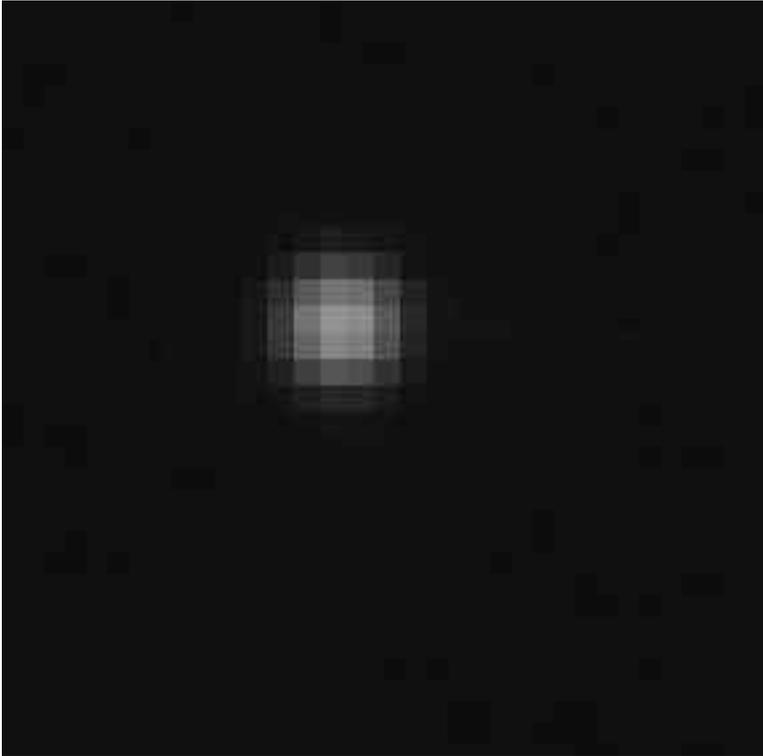
Figure 1: Image of BCAM light source taken with BCAM that had received a dose of 400 Gy ionizing radiation.
