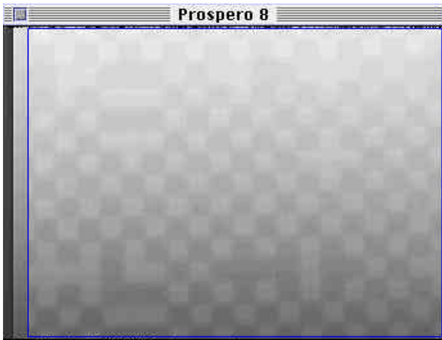
Figure 1: An image captured from a CCD that took 9.1 Tn. The exposure time was 2 ms. The pattern is the shadow cast by a rasnik mask held up against the CCD. The squares are 170 \mu\text{m} wide.
