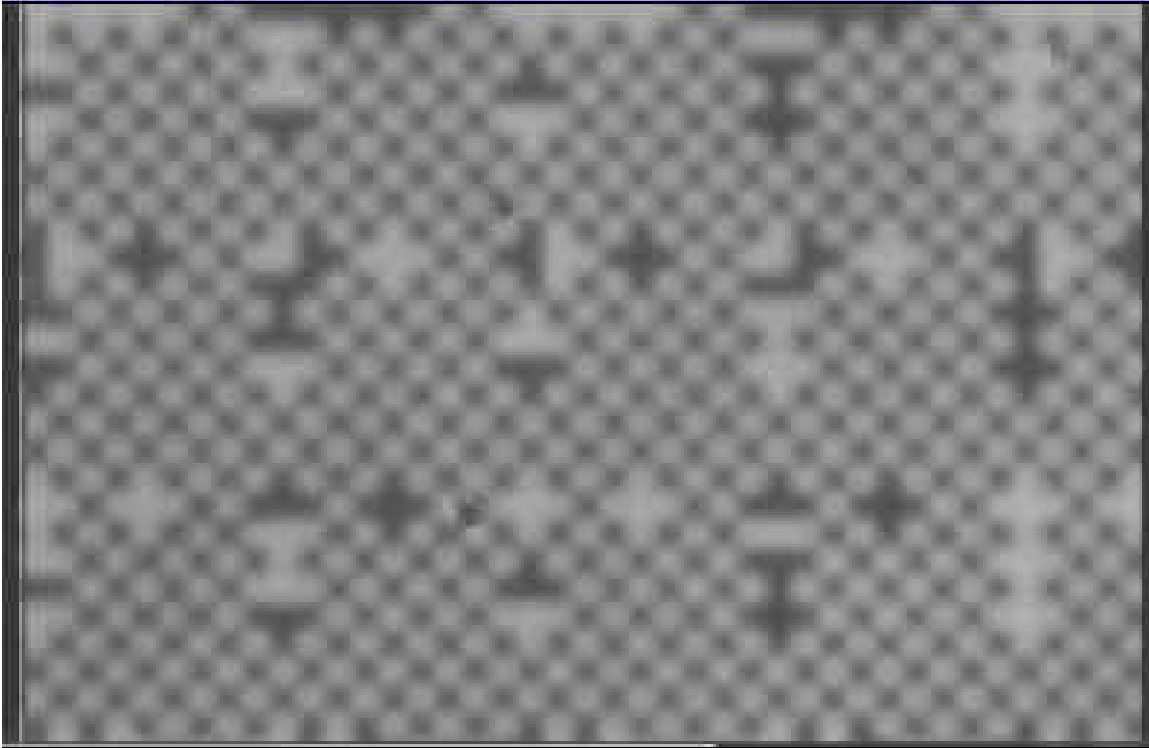
Figure 3: A Pixel CCD RASNIK Image (25-mm lens aperture)
