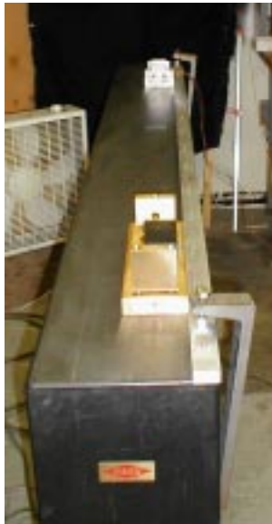
Figure 9: Picture of the granite bar and BCAM setup used to obtain the relative rotation of this uncalibrated BCAM about the longitudinal axis of the global coordinate system.
