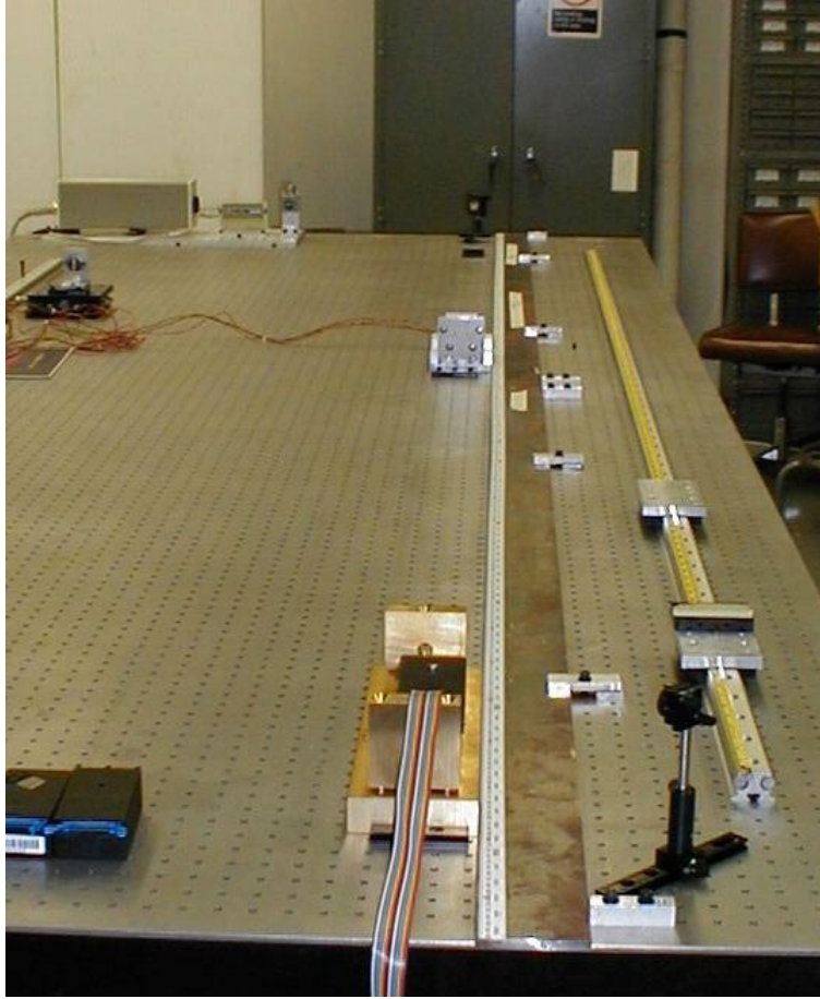
Figure 6: Picture of the optical table on which the calibration data were taken. A BCAM is mounted in the roll cage in the 0^\circ orientation in the foreground, the source block is middle of the picture, and the laser for the interferometer may be seen at the upper left.
