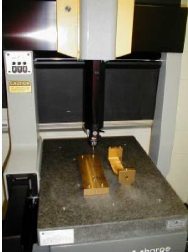
Figure 4: Brass roll cage (right) and base (left) being measured by the coordinate measuring machine (CMM). The BCAM views through a hole in the end of the roll cage which can be seen clearly in this picture.
