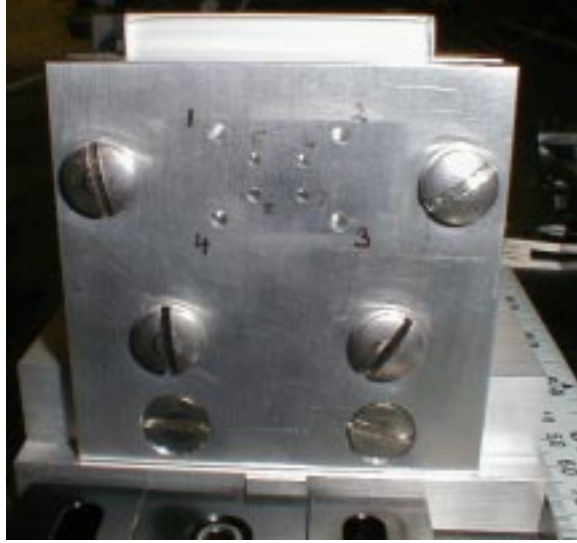
Figure 7: Front view of the source block showing the rectangular array of conical source holes.
