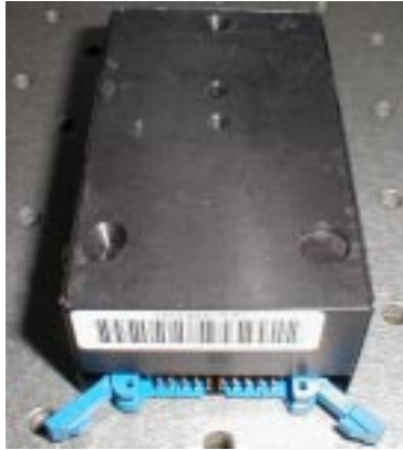
Figure 2: The underside of a BCAM, showing the mounts for the three balls: cone at upper center, slot at lower left, and plane at lower right.
