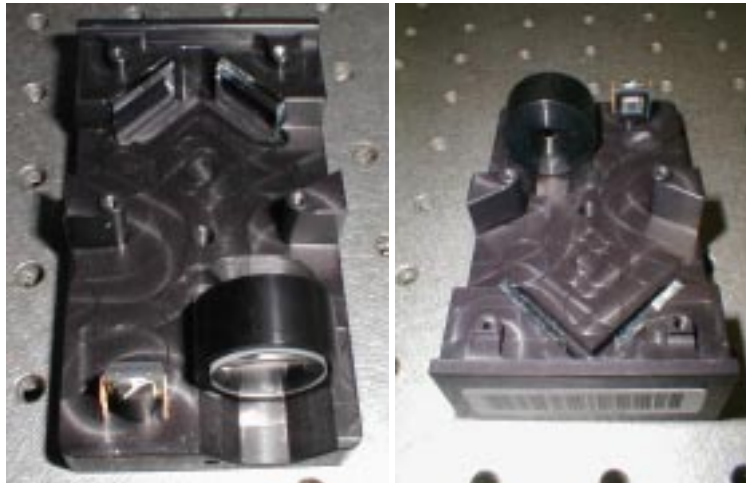
Figure 1: These are pictures of a BCAM with its cover (and IR filter) taken off and electronics removed. In the left picture, the light proceeds through the lens at the lower right, reflects off the mirrors at the top, and is recorded by the CCD at the bottom left. In the right picture, one may see the aperture behind the lens at the upper left, the two mirrors at the lower left and right, and the front of the CCD at the upper right. The screw holes on the optical table are placed at 1 inch (25.4 cm) intervals to give a sense of scale.
