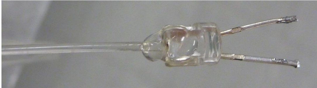
Figure: FH1011 LED secured to one end of an ESKA 1000 micron fiber with two-part optical epoxy.
