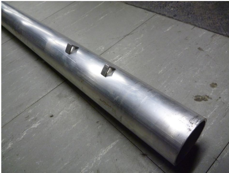
Figure: Two tube mounts resting atop one end of the LGT. The fiber end will be attached to the inside of the apex each forms.
