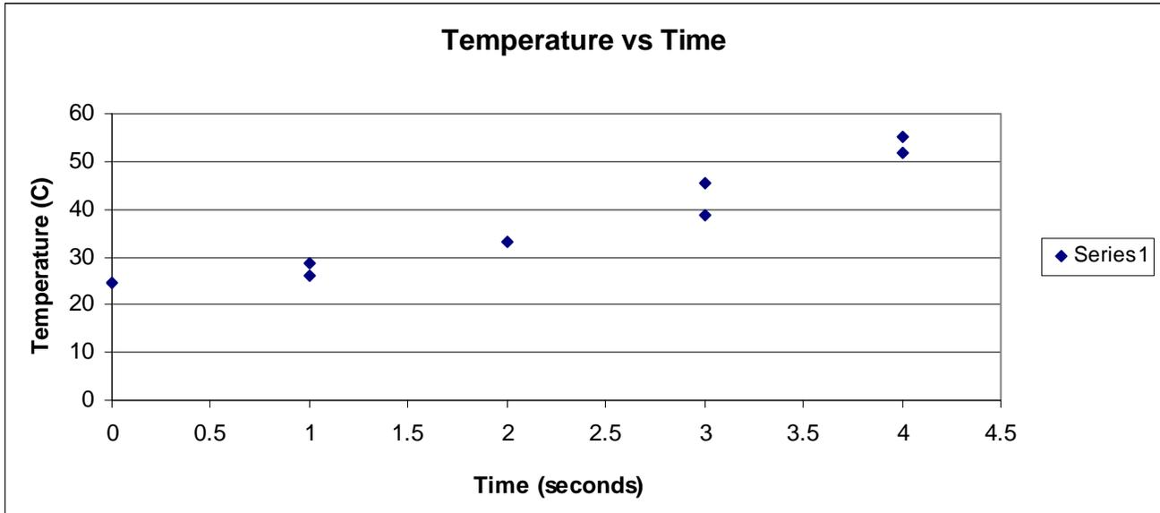
Figure 4: Temperature (C) vs. time. Temperature sensor saturated at 55 degrees C.
