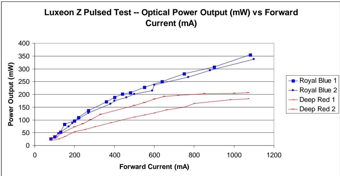
Figure 5: Optical Power Output vs Forward Current.
