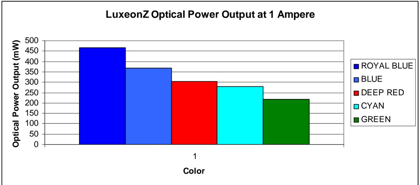
Figure 1: Optical Power Output at 1000mA versus Color. Power measured with a SD445 Photodiode, 15V reverse bias, and 100Ohm Resistor. Datasheet for the SD445 can be found at [1].
