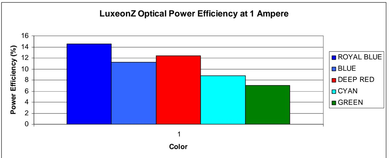
Figure 2: Optical Output Power divided by Electrical Power input vs. Color.
