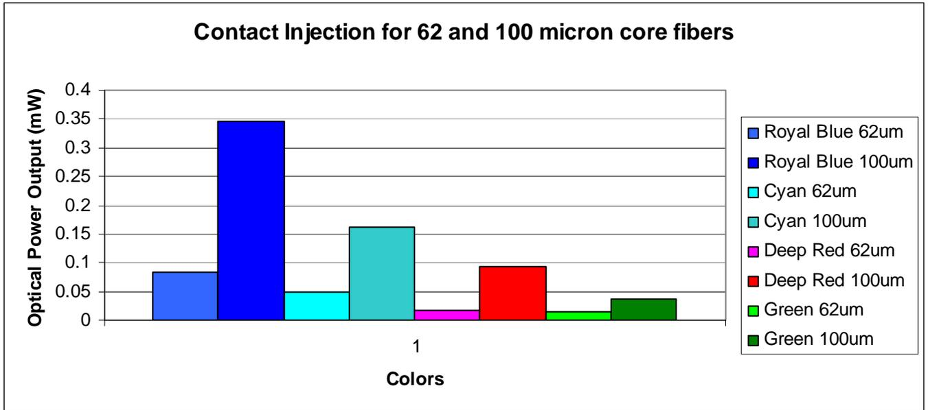
Figure 3: Optical Power Output through fiber vs. Color & fiber core diameter.
