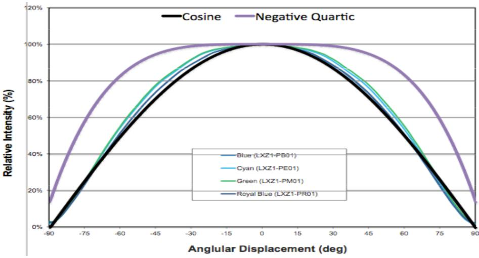
Above shows the two curves fit over the data sheet graph of intensity versus angular displacement for different Luxeon-Z LEDs, which shows is cosine was a good fit for the intensity vs angular displacement of these LEDs.
