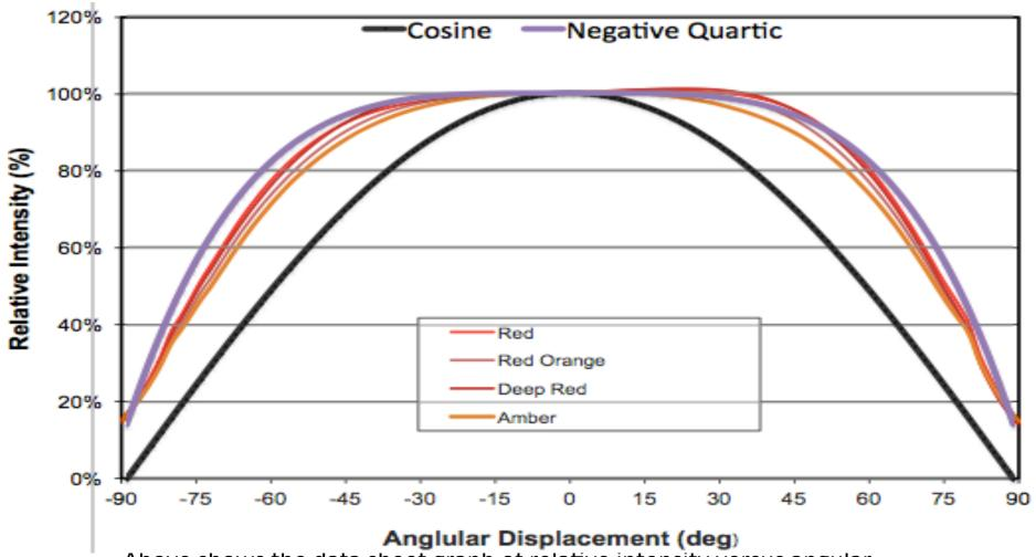
Above shows the data sheet graph of relative intensity versus angular displacement for different colored Luxeon-Z LEDs. Overlapped is a cosine function and a negative function of theta<sup>4</sup>. The cosine has a clear forward bias, which was a source of error in intensity calculations.
