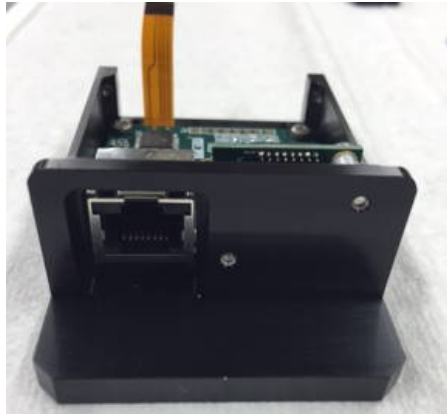
Figure 8: Make sure RJ-45 sits properly in the base as shown.
