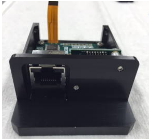
Figure 6: Make sure RJ-45 sits properly in the base as shown.
