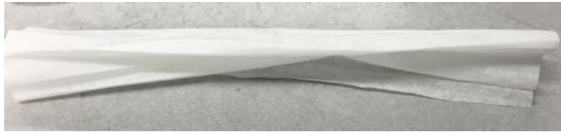
Figure 12: Folded wipe to be used to clean the CCD.
